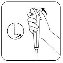
**Reverse Deflection** Level Up = Tip Down Level Down = Tip Up
