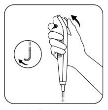
**Standard Deflection** Level Up = Tip Up Level Down = Tip Down
