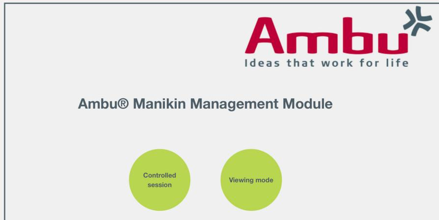
Start the training device and connect your end device with the training device. Open the browser and enter <http://Ambu.login> or [192.168.1.1](http://192.168.1.1) into the address line to get to the start screen of the Ambu Manikin Management Module. Finally, select the button "Controlled session".
