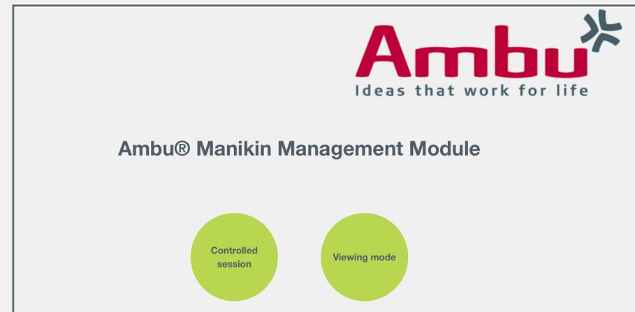
Enter **http://Ambu.login** or **192.168.1.1** into the address line to get to the start screen and select this time the button "Viewing mode".
