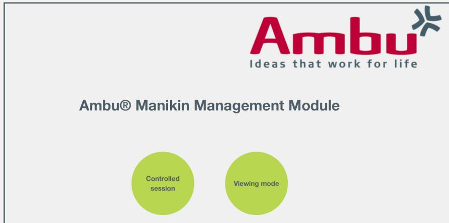
Start the training device and connect your end device with the training device. Open the browser and enter **http://Ambu.login** or **192.168.1.1** into the address line to get to the start screen of the Ambu Manikin Management Module. Finally, select the button "Controlled session".
